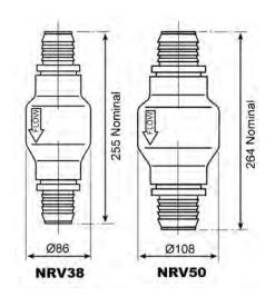
When part of an overboard system valves must not be installed below the waterline.
