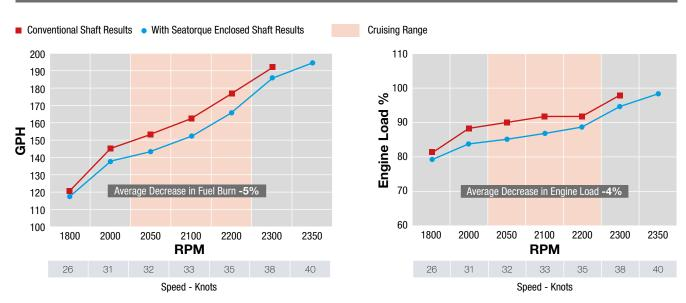
Test Boat Specifications: LOA - 64ft Displacement - 109,000lbs Engines: MTU 16V2000M91 2000hp
