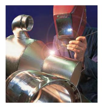
Halyard products including stainless steel risers, water injection spray heads, exhaust transom outlets, supports, high temperature GRP silencers and separators, tube and connectors, marine exhaust hose, silicone hoses and bellows are designed and manufactured in-house at our UK manufacturing facilities.
