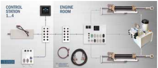
— CAN-BUS CONNECTION ••• ELECTRIC HARNESS — HYDRAULIC CONNECTION
