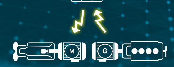
This is a versatile arrangement allowing electrical generators to be installed anywhere in the hull. These generate electricity which is used to power electric motors, with batteries acting as a buffer of energy. The generators charge the batteries during low power demand. During high demand the batteries "top-up" power to the motors, leading to more constant diesel power and increases in efficiency.
